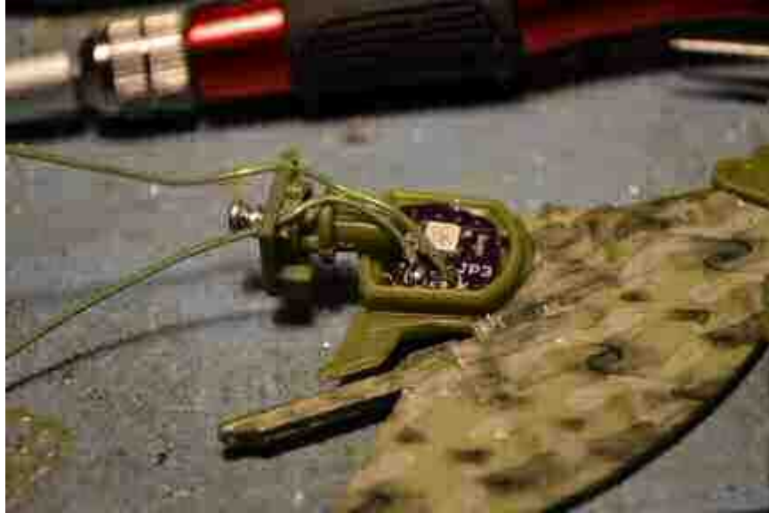
Figure 19. Solder Wire to the Wing LED board
