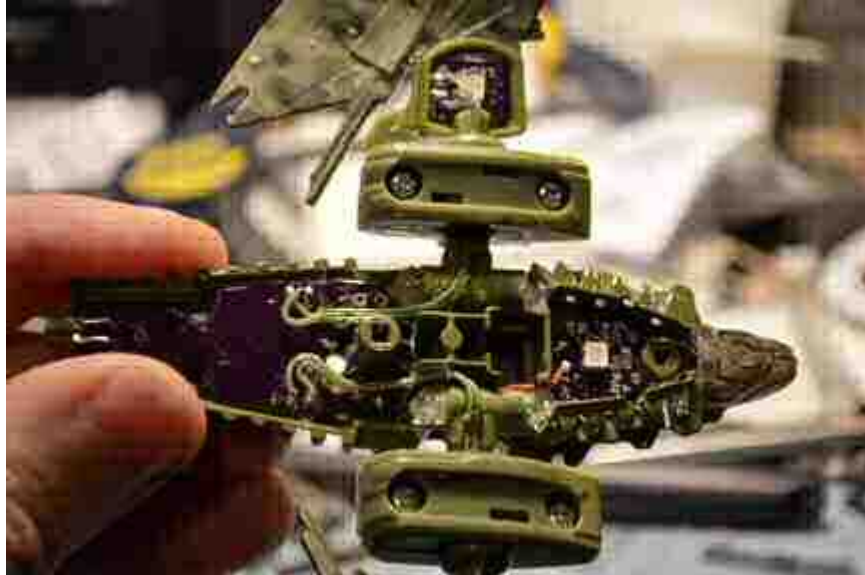
Figure 23. Wire WingLEDs to Body board
