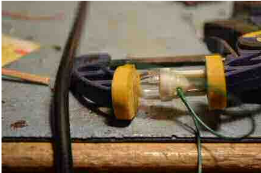
Figure 35. Epoxy Lens to LED base
