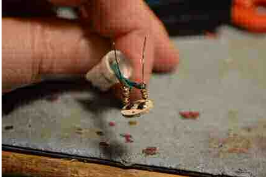
Figure 34. Solder GI wires to LED leads
