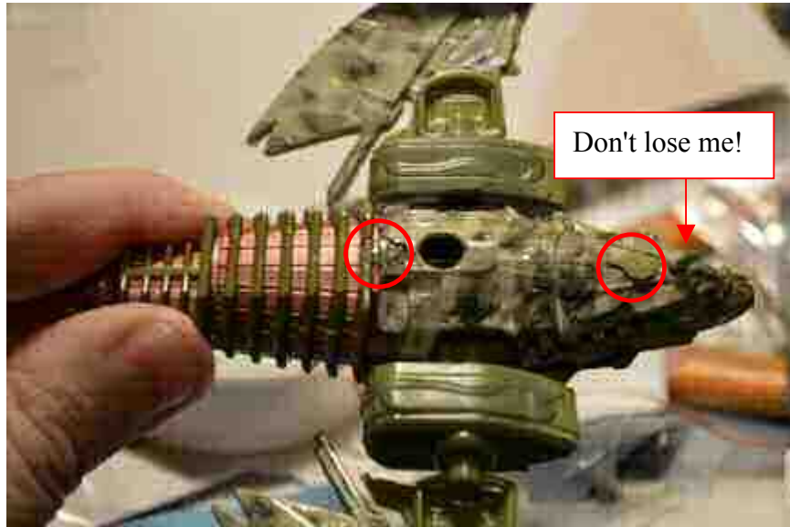
Figure 4. remove screw hiding plugs
