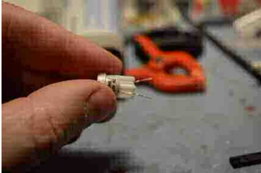
Figure 32. Straighten LED leads to remove base
