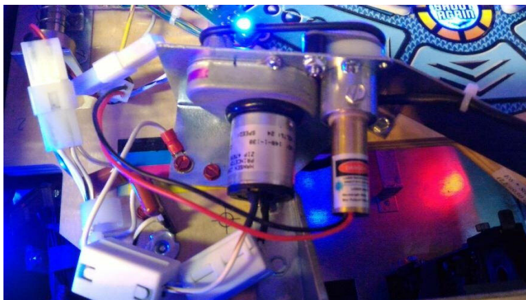
Figure 4 New Laser Module installed with insulator
