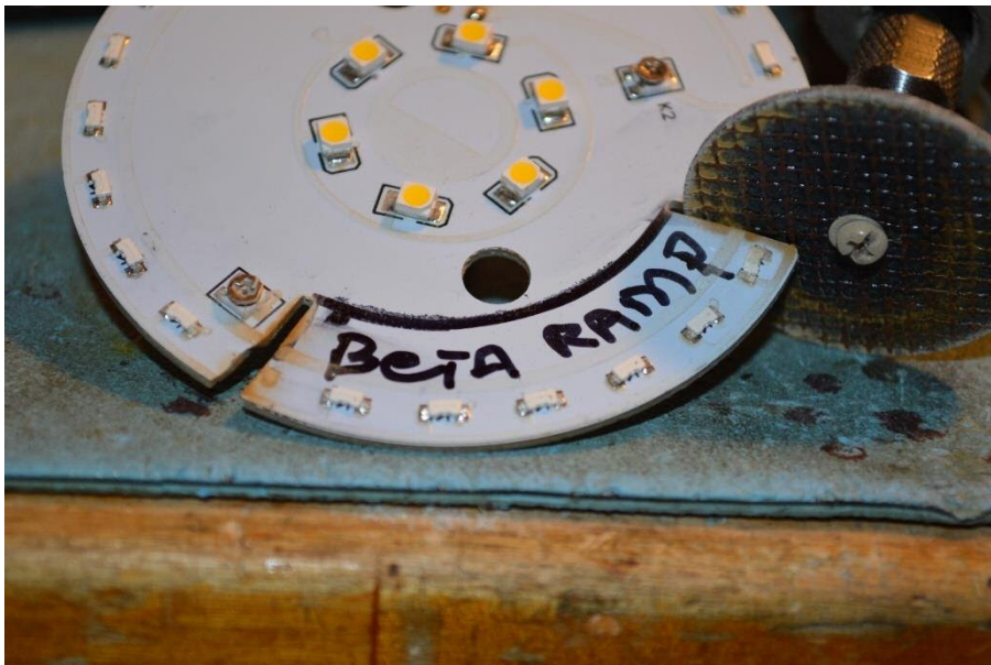
Figure A.1.25 Cut opposite side
