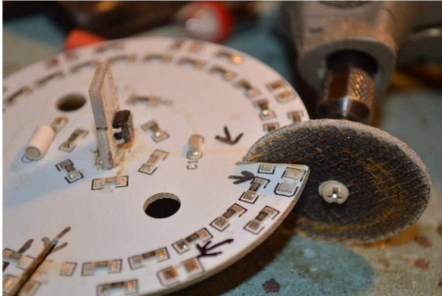
Figure A.1.24 Use Cutoff Wheel protecting C1 trace identified
