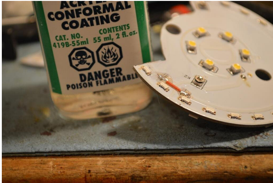
Figure A.1.38 Insulate bridged trace connections
