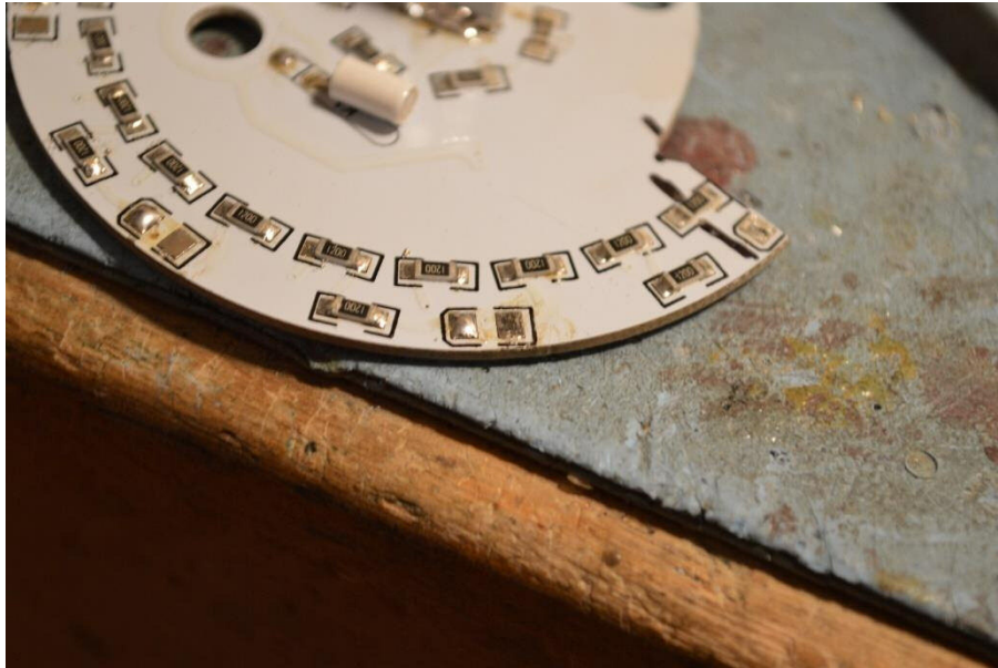
Figure A.1.35 Add solder to Cathode pad for LED installation
