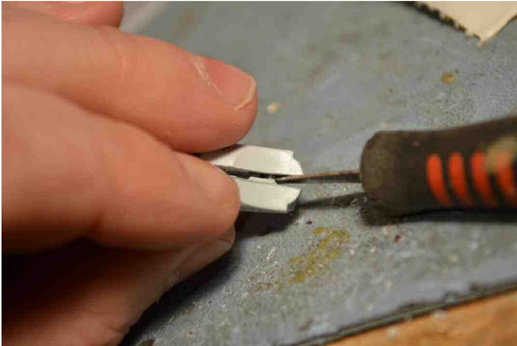
Figure 16. Pry Halves apart using xacto blade.
