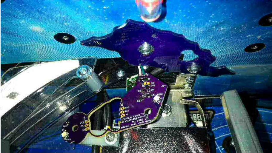
Figure 11 Thread -67 JGI into warp ramp slot but over the warp ramp
