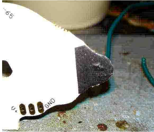
Figure 6 Trim wire/solder flush with PBA
