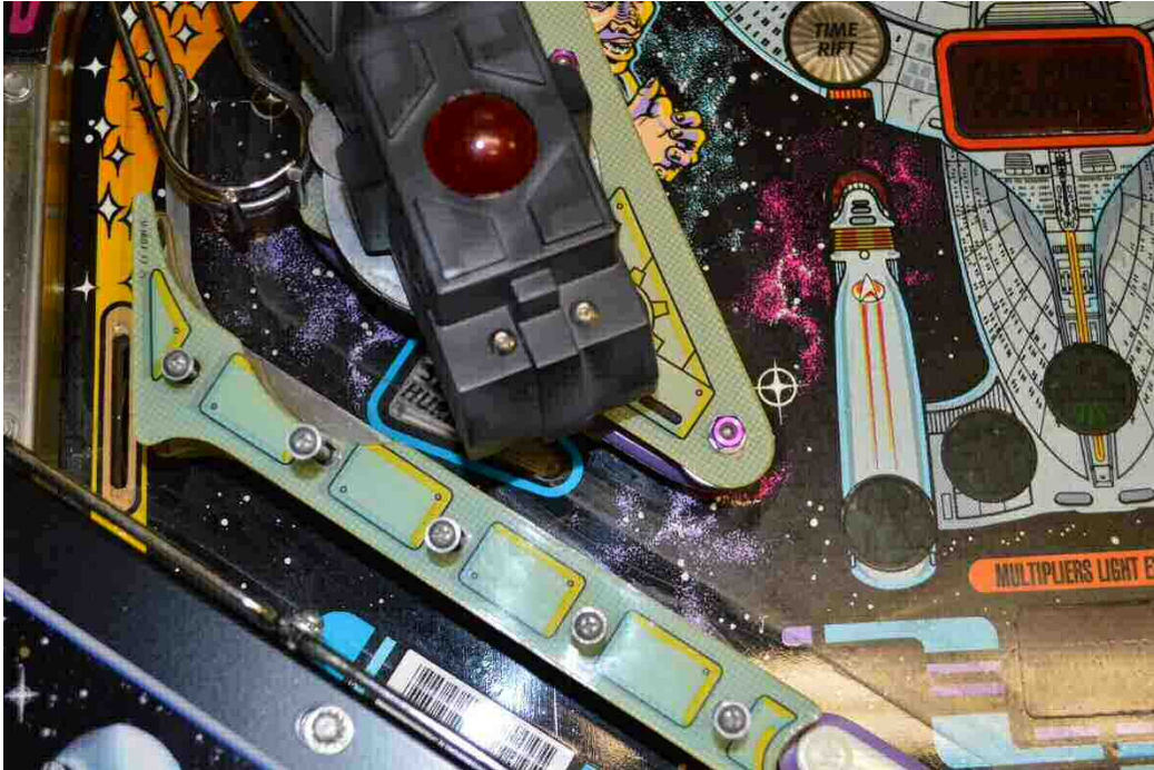
Figure 0.4 loosen Philips head screws
