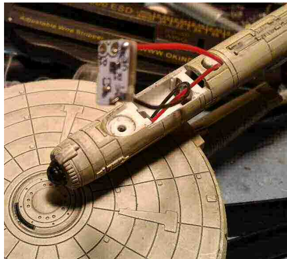
Figure 17 Solder VCC & SW to VE & V- on BAT board
