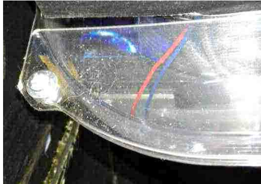
Figure 27 GI wires under beta ramp behind backboard
